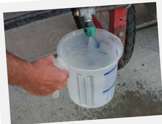
Figure 23. Capturing nozzle discharge
